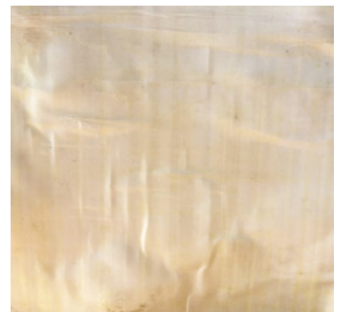
ASL GRP's Legion Polyethylene rear of tested panel -clear pass.
