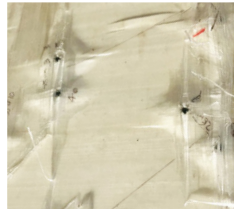
ASL GRP's tested Legion Polyethylene shot face
